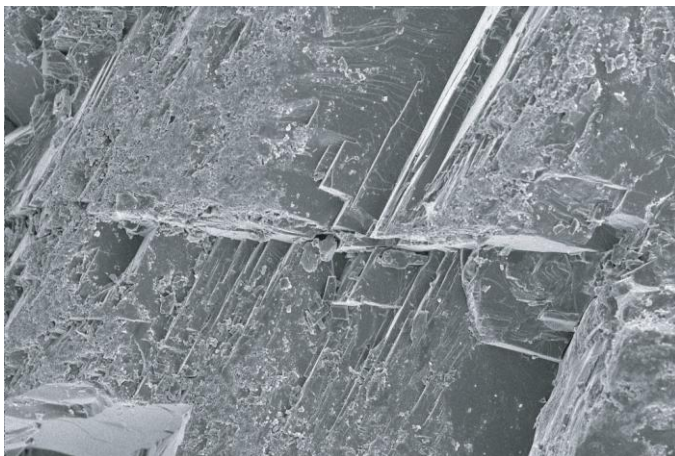
SEM image of stepped fractures on broken surface of rough ruby from Longido, Tanzania
